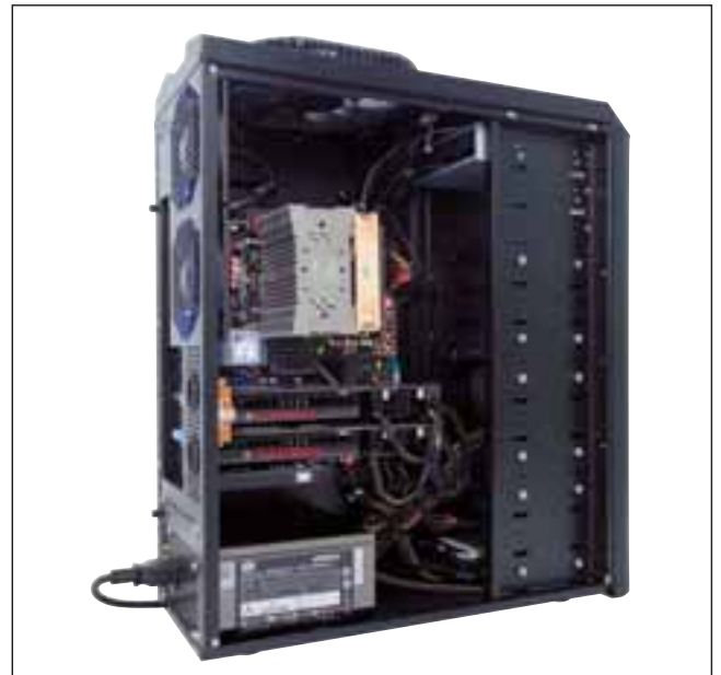
The Fusion is cooled by a huge third-party Noctua cooler
